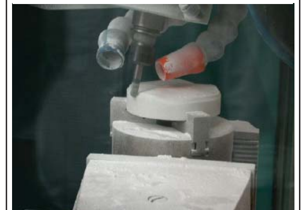
Lamp body produced from Thassos Marble. Top - digital model, Bottom - lighting body's machining at the LithoCerm1
